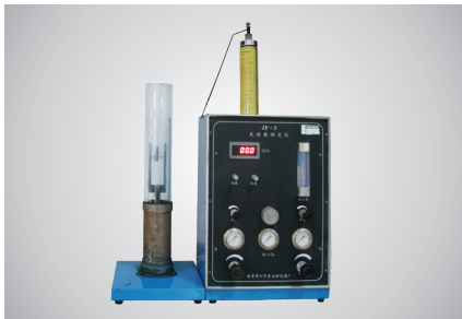
氧指数测定仪 Oxygen index tester
