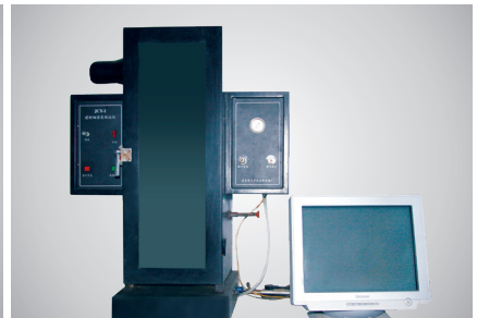
烟密度测试仪 Smoke density tester
