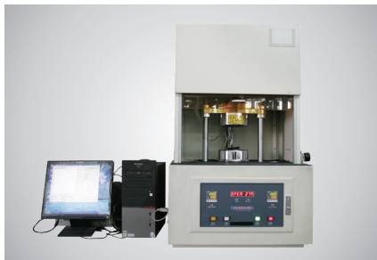
门尼粘度仪 Mooney viscometer
